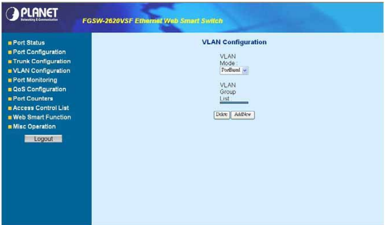
Figure 4-13 Port-based VLAN Configuration Web Page screen
